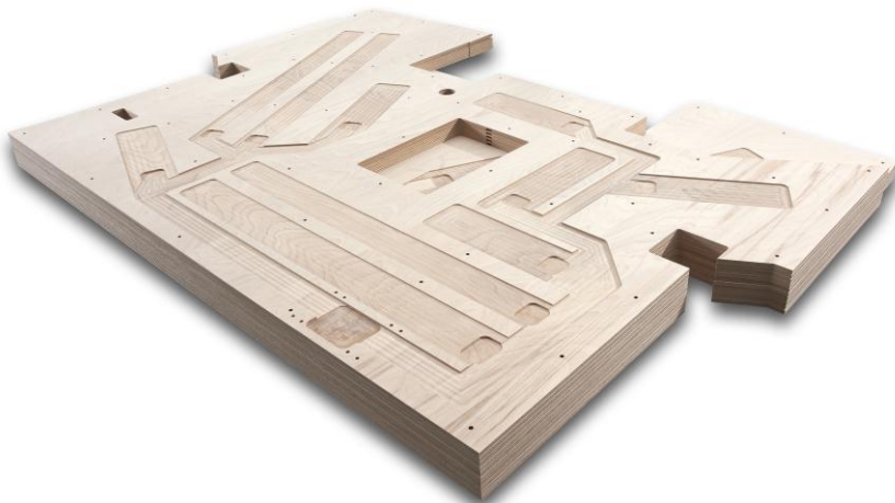
Image 1 CNC-machined and ready-to-install floor panel for the train driver cabs
